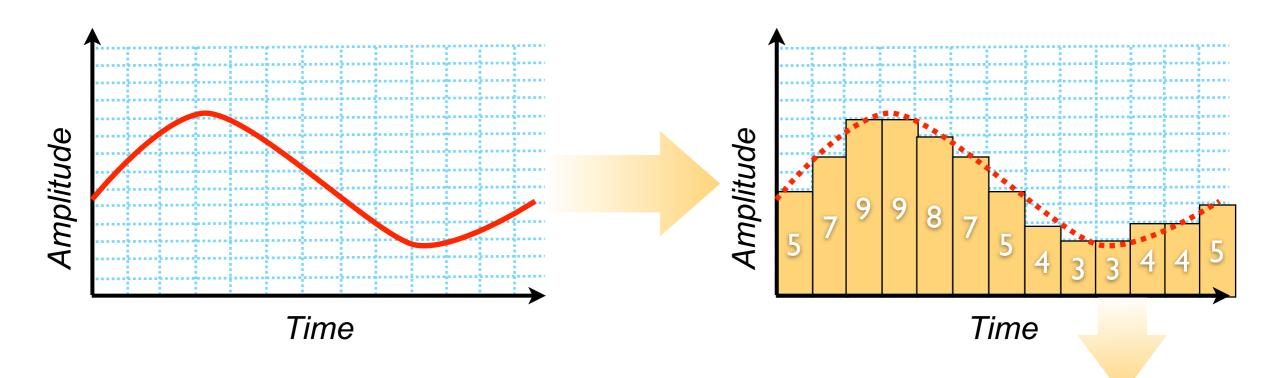
Any analogue signal can be represented digitally: sample the signal at a suitable rate, quantise to nearest allowable discrete value, and convert to digital representation
