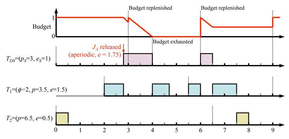
Add the deferrable server, scheduled according to the rate monotonic priority, but with the budget consumption and replenishment rules affecting its execution time
