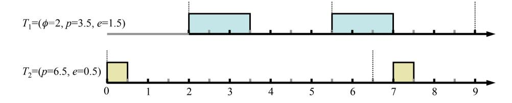
Periodic tasks  $T_1$  and  $T_2$  are scheduled according to the rate monotonic algorithm
