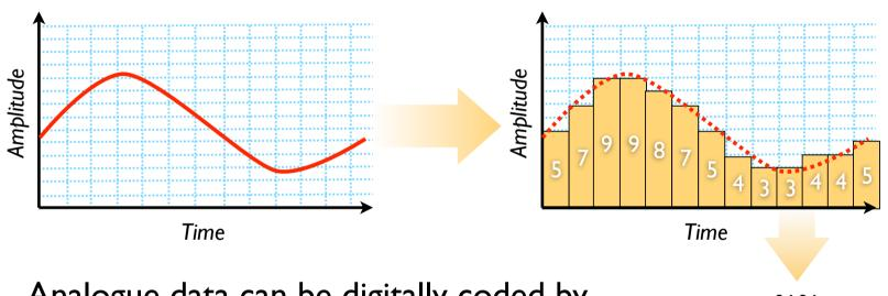
Analogue data can be digitally coded by sampling at a suitable rate, quantising to the nearest allowable discrete value, and then converting to digital representation (PCM)
