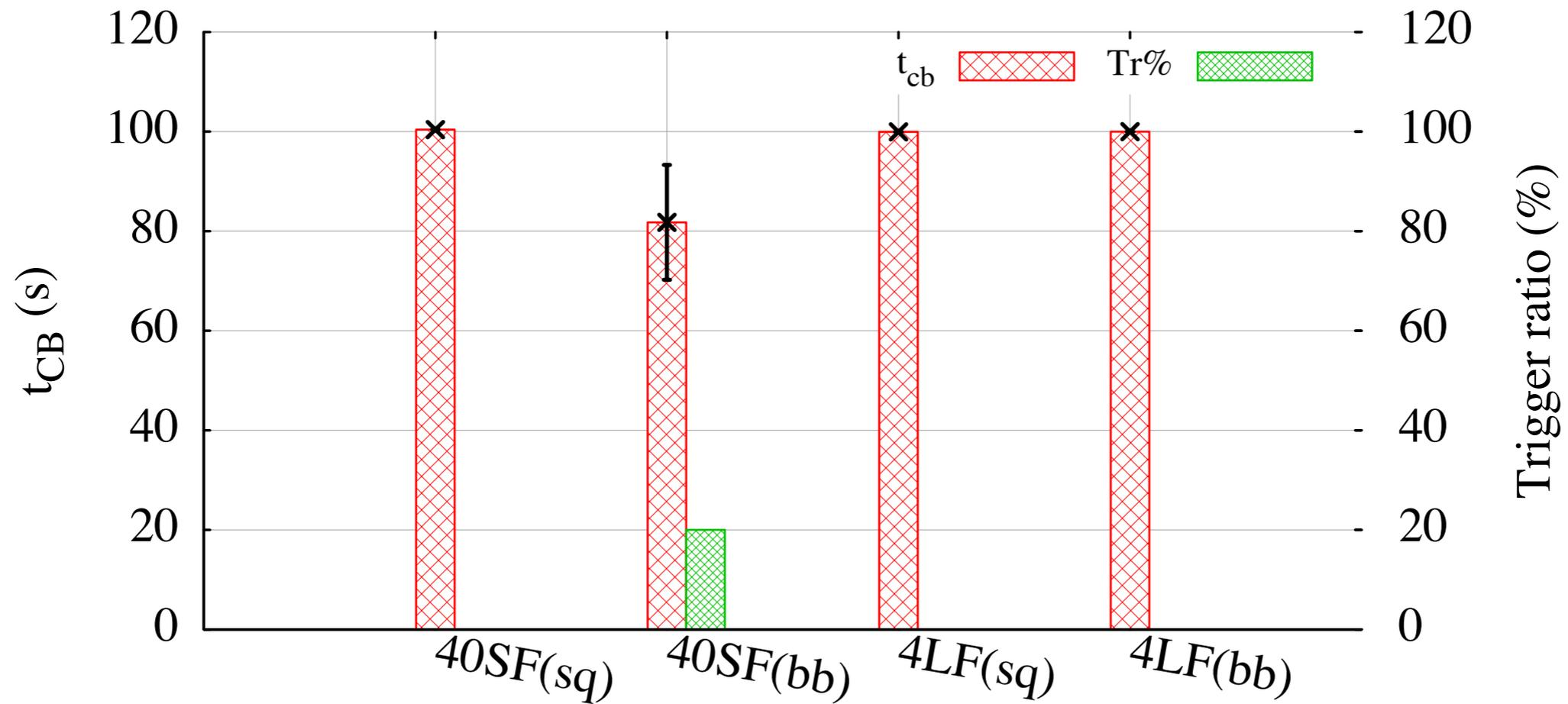
Buffer bloated queue fills up the queue. Bursty losses are detected at the endpoints which triggers the circuit breaker.
