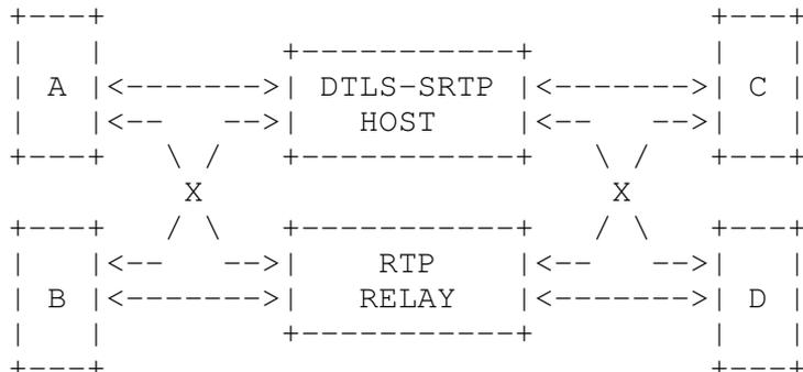
Figure 3: DTLS-SRTP host and RTP Relay Separated
