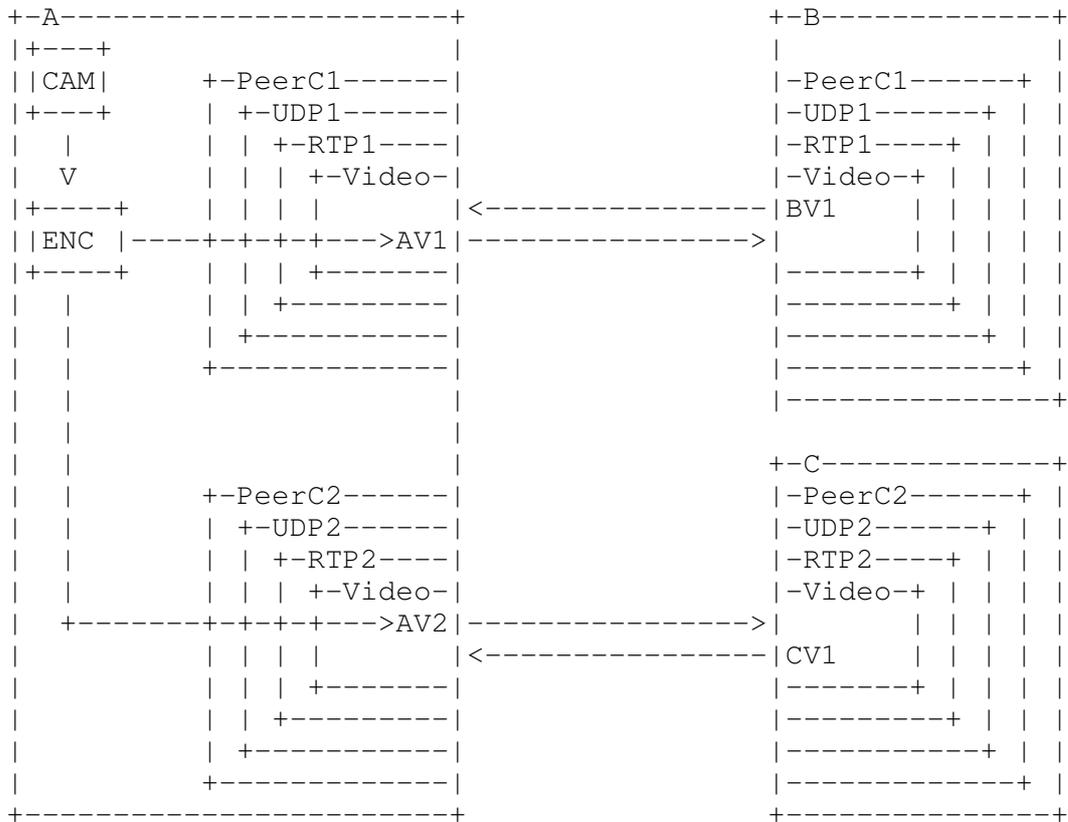
Figure 10: Single Encoder Multi-Unicast Setup
