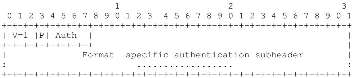
Figure 3: Format of the authentication data in the SAP header
