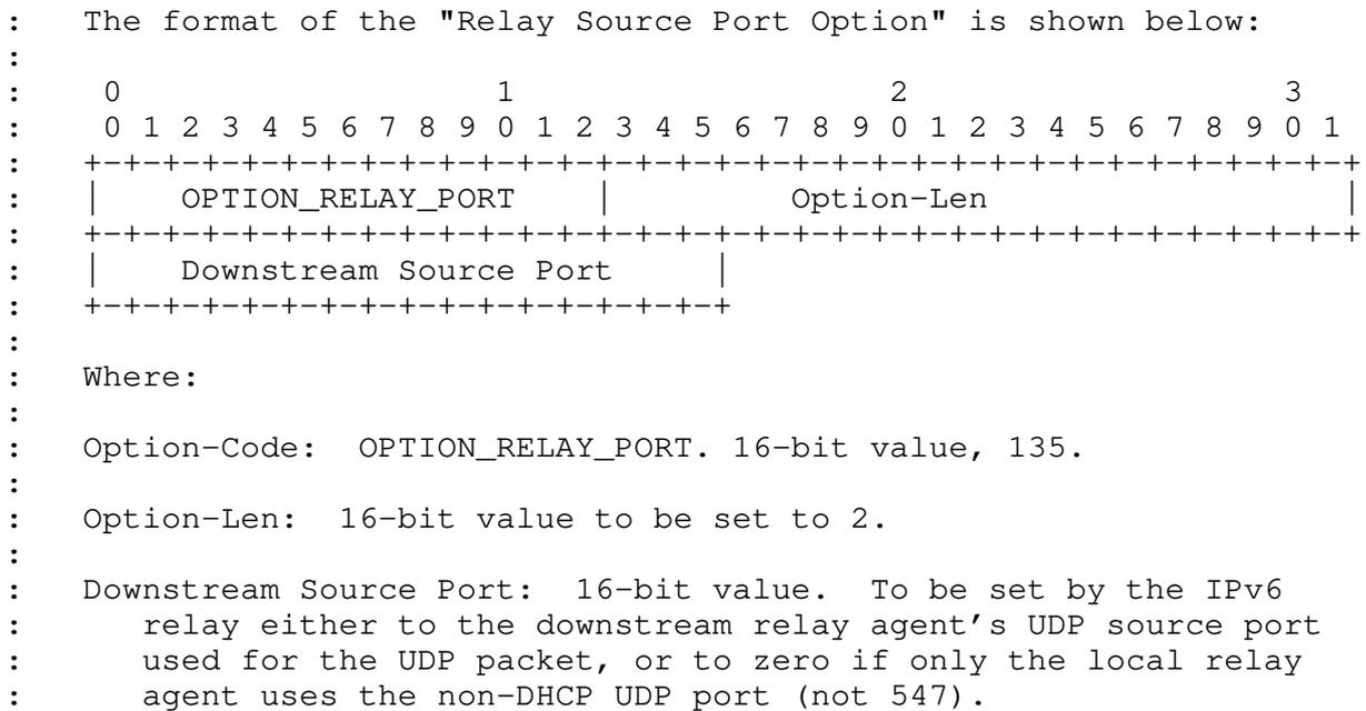
Figure 3: DHCPv6's Relay Source Port Option (from [RFC8357])
