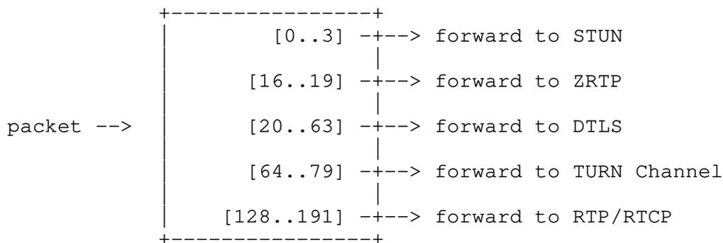
Figure 3: The DTLS-SRTP receiver's packet demultiplexing algorithm.
