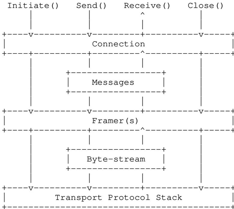
Figure 1: Protocol Stack showing a Message Framer
