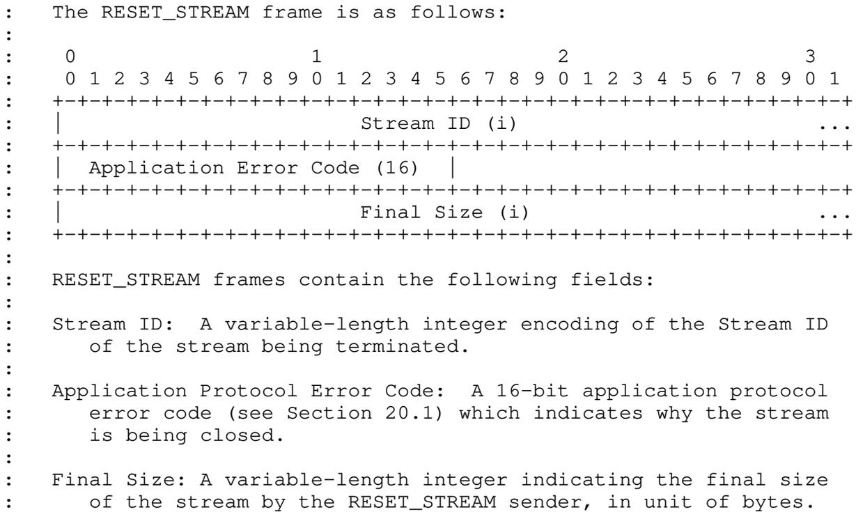
Figure 2: QUIC’s RESET\_STREAM frame format (from [QUIC-TRANSPORT])
