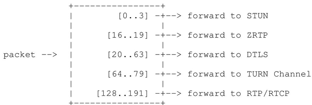
Figure 1: DTLS-SRTP receiver's packet demultiplexing algorithm.
