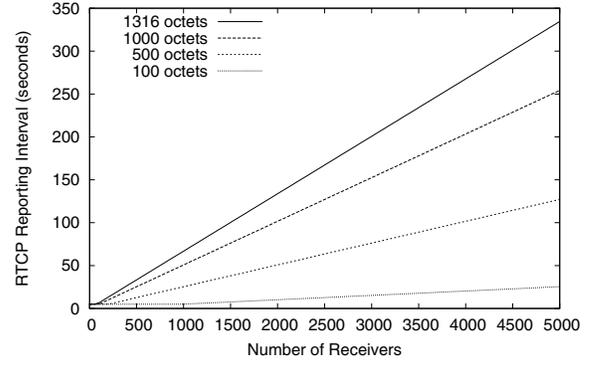
Fig. 4. Increase in RTCP reporting interval with increasing packet size (from 100 to 1316 octets) and number of receivers. Media bandwidth is 4.2 Mbps.
