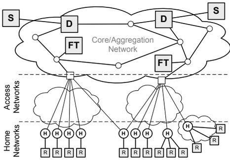
Fig. 2. Intradomain IPTV distribution and monitoring architecture.
