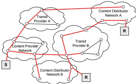
Fig. 1. Transit and distributor networks connecting the content servers and receivers.
