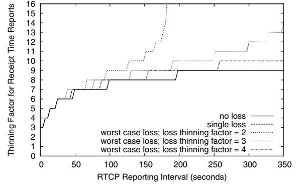
Fig. 5. Required  $T_r$  with increasing group size for the FT  $\leftrightarrow$  R RTCP session. RTCP packet size is 1316 octets.
