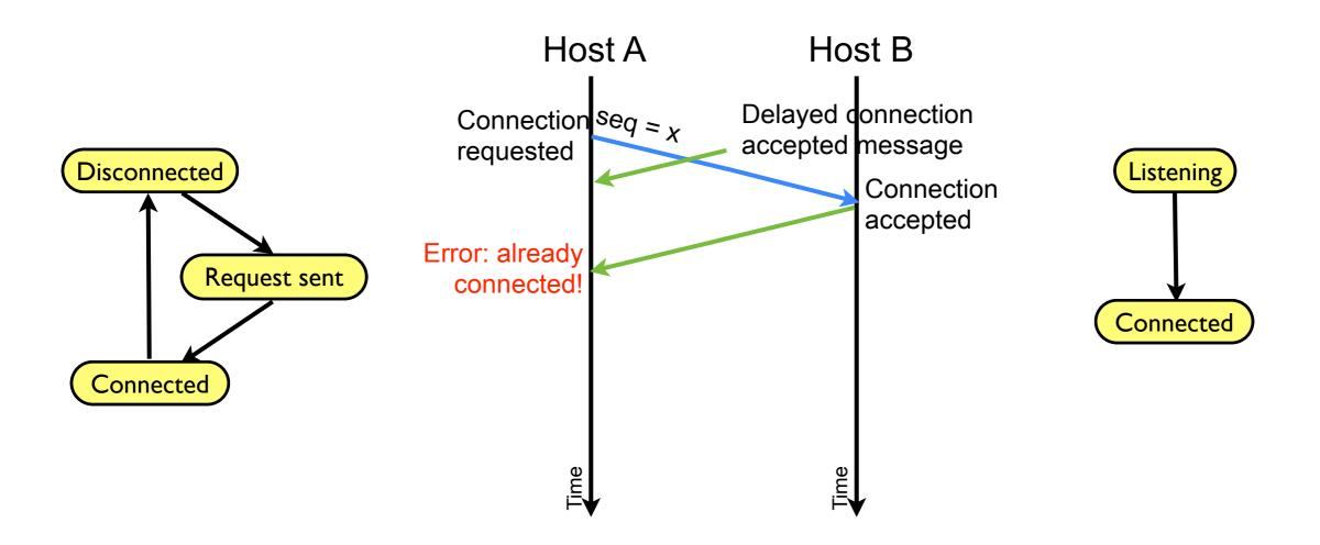
Solution for robust connection establishment: use a three-way handshake
