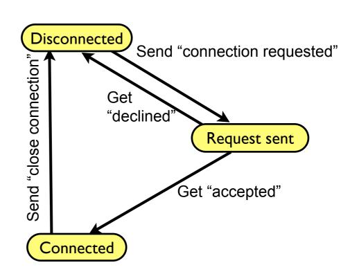
Example: partial state machine for opening and closing a connection
