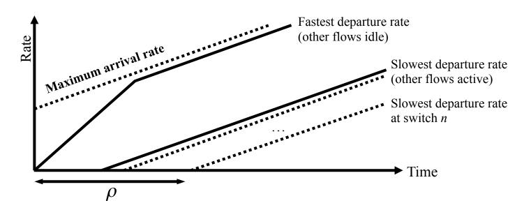
• Making worst case assumptions, maximum arrival rate at switch *n* is slowest departure rate at switch *n*-1; 1 unit of delay added due to non pre-emption at each hop
