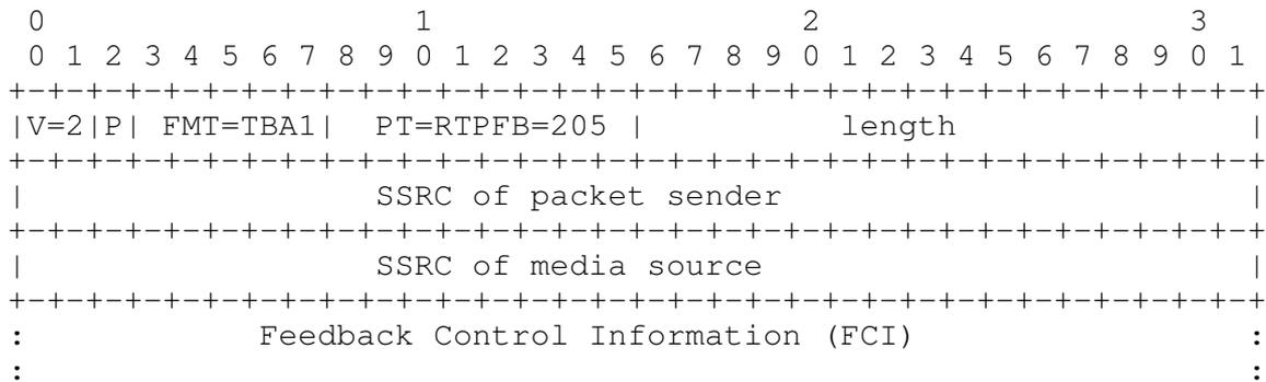
Figure 1: RTP/AVPF Common Packet Format for Feedback Messages
