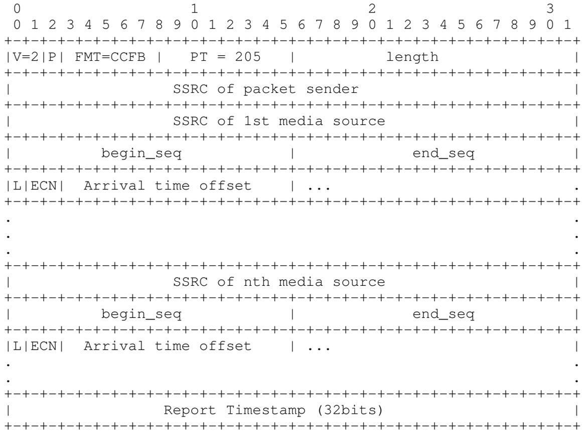
The first 8 octets are the RTCP header, with PT=205 and FMT=CCFB specifying the remainder is a congestion control feedback packet, and including the SSRC of the packet sender. (NOTE TO RFC EDITOR: please replace CCFB here and in the above diagram with the IANA assigned RTCP feedback packet type)
