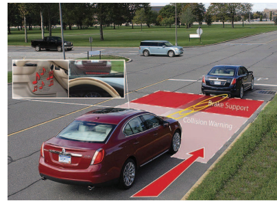
Fig. 1. Collision Warning with Brake Support. Image provided by the Ford Motor Company, USA under Creative Commons Attribution 2.0 Generic license.
